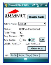
• **Enable/Disable Radio**: Enables or disables the radio. This is a toggle button; when the radio is enabled, this button reads *Disable Radio* and when the radio is disabled, the button reads *Enable Radio*.
